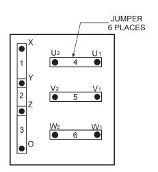
Figure 16. Voltage Change-Over Board 240V Configuration
